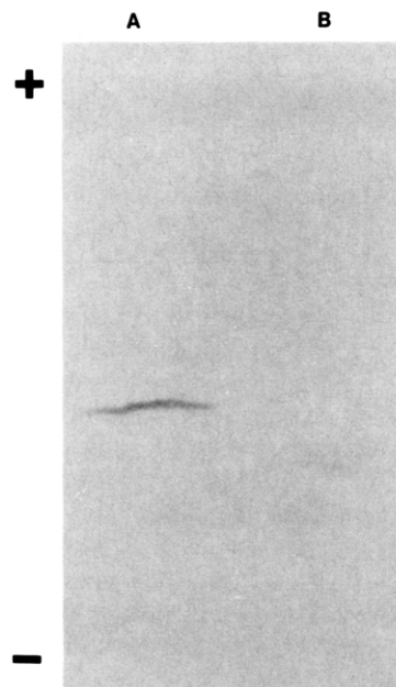
FIGURE 3: Paper print of thin-layer isoelectric focusing of natural bovine insulin (A) and synthetic [Leu 19 -A]insulin (B) in a 1:1 mixture of pH 3–10 and pH 4–6 ampholytes on a 20-cm separation distance. Focusing was at a constant power of 8 W for 4 h.
